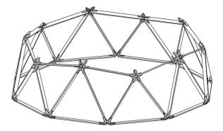
14. Continue to install the hubs and struts per the colors, fastening along the way. When necessary, support any hanging struts until both ends are supported so undue forces are not put on the connectors which may bend or break them. The true strength of a geodesic dome comes from the completed structure and care must be taken until all pieces are in place.
