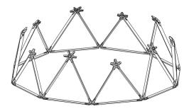
13. Insert the correct horizontal struts between the newly installed hubs and fasten to form the 2<sup>nd</sup> horizontal row.
