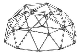
15. Once you've started to add the final 5 struts, fasten the "keystone" hub to the first board and add each additional strut fastening along the way until the dome frame is completed. NOTE – On HD Pipe Dome Kits, the Keystone hub comes in two pieces and should be assembled around the top 5 struts then bolted through the center as well as fastened to the pipes making sure they are butted up tight.
