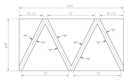
This guide outlines the general procedure of cutting the panel triangles used for a 3v Dome. Always account for overlap on the struts and an expansion gap between panels. As a general rule, the panel side dimension should be 5-1/2" longer than the strut that it would be covering. Always check prior to cutting.
